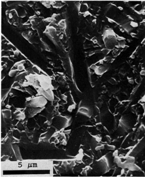
Fig. 9. SEM micrograph fracture surface of the toughest monolithic ceramic.
